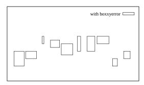
The box width and height are determined from the x and y errors in the same way as they are for the **xyerrorbars** style — either from xlow to xhigh and from ylow to yhigh, or from x-xdelta to x+xdelta and from y-ydelta to y+ydelta, depending on how many data columns are provided.
