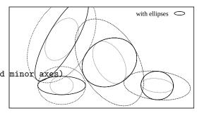
If only two input columns are present, they are taken as the coordinates of the centers, and the ellipses will be drawn with the default extent (see **set style ellipse** (**p. 205**)). The orientation of the ellipse, which is defined as the angle between the major diameter and the plot's x axis, is taken from the default ellipse style (see **set style ellipse** (**p. 205**)).
