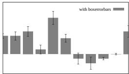
The box height is determined from the y error in the same way as it is for the **yerrorbars** style — either from y-ydelta to y+ydelta or from ylow to yhigh, depending on how many data columns are provided.
