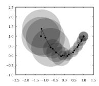
By default a full circle will be drawn. It is possible to instead plot arc segments by specifying a start and end angle (in degrees) in columns 4 and 5.
